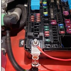
Attach the ground (black) ring terminal to the ground stud located near the fuse box using a 10mm socket.
